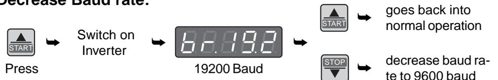
After changing of the baud rate the display of the operator goes into normal operation.
