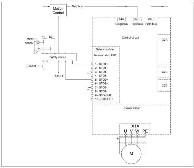
When pressing the emergency stop unit the drive is stopped with a deceleration ramp via input X2A.13 (I3).
