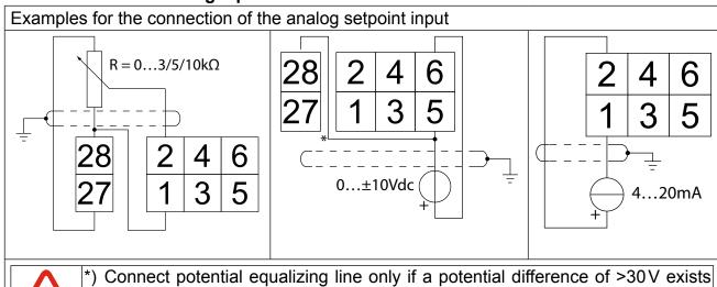
between the controls. The internal resistance is reduced to  $30\,k\Omega$ .
