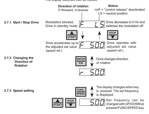
2.7.4 Leaving the "Drive Mode" To exit the Drive Mode the inverter must be in status "stop" (Display noP or LS). Press the "FUNC and ENTER" keys simultaneously for about 3 seconds to leave the Drive Mode. The CP-parameters appear in the display.
