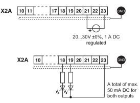
**1.1.7 Relay Outputs** In case of inductive load on the relay outputs, protective wiring must be provided (e.g. free-wheeling diode, see figure in section 1.2.6)!
